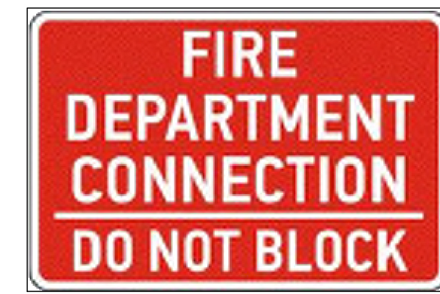
12" X 18" 0.63" WHITE RUST FREE ALUMINUM 2" WHITE LETTERING ON RED BACKGROUND FIRE DEPARTMENT SIGNAGE DETAIL SCALE: NTS
